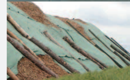
Passive drying of wood chip Semi permeable fabric coverings have been successfully used to aid woodchip drying at several sites around the UK. South Yorkshire Forest Partnership
