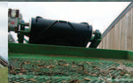
Screening wood chip to improve chip quality Bristol City Council installed wood chip boilers at several locations using chip arising from management of the city's trees as fuel. With unscreened fuel the boilers were liable to smoke and malfunction. Once screened chip was made available boiler performance and reliability improved and fuel consumption reduced. BioRegional Development Group
